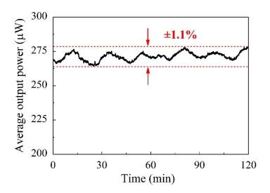
Fig. S3 Average-output-power stability of the laser oscillator over 2 hours.
