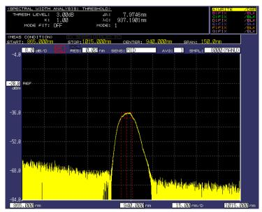
Fig. S2 Frequency-doubled spectrum using a 1-mm-long PPLN crystal.
